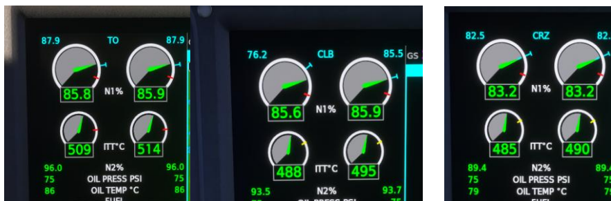
EICAS showing thrust rating modes
